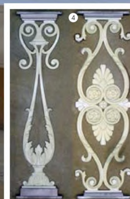
Stampo in resina per prototipo in alluminio Resin mold for aluminum prototype
